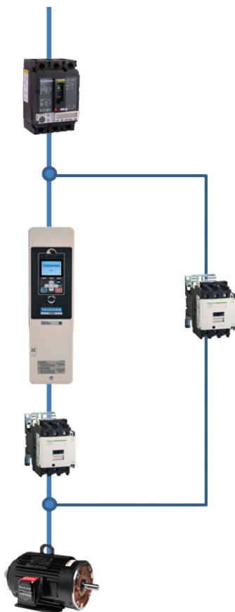
Figure 12: Two-contactor bypass setup
