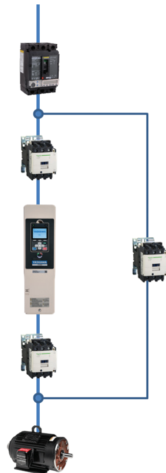
Figure 13: Three-contactor bypass setup
