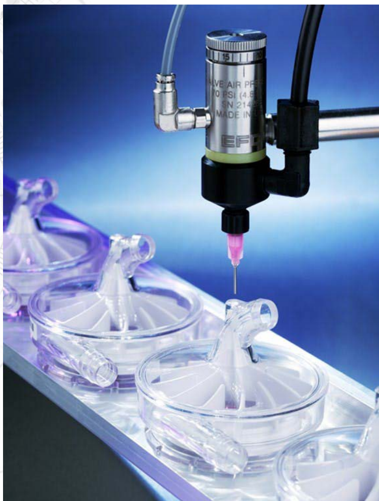
Needle valves are an essential technology for enabling manufacturers to build smaller medical device components—empowering organizations to deposit microdots as small as 150 \mu\text{m} (0.15 mm) (0.006 in.) diameter. Nordson EFD
