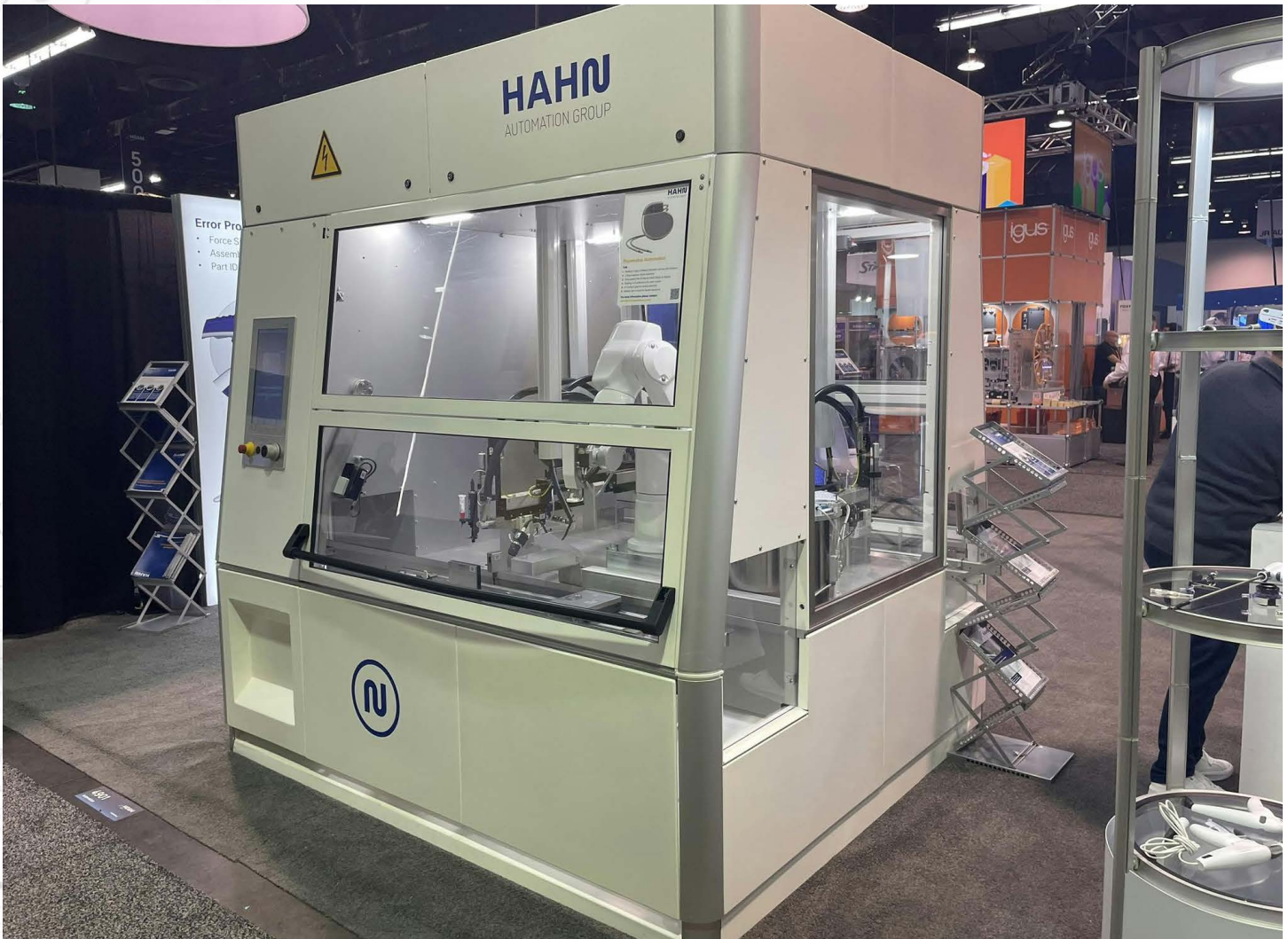
Hahn Automation Group's cell features a multi-carrier magnetic system as well as a flexible link conveyor system. The advanced motion control demo showcases flexibility, precision and efficient use of floor space. Hahn Automation Group
