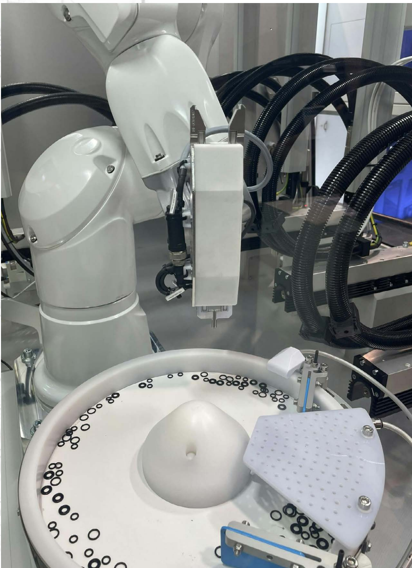
A dual-sided demonstration depicts both demo syringe assembly and pacemaker assembly. This image highlights the pacemaker assembly side, where O-rings of varying sizes are loaded into a FlexiBowl feeder.
