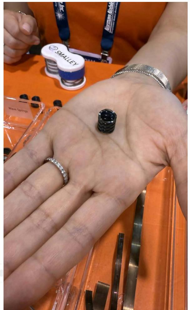
Smalley is preparing to launch a high-force spring. Called a nested crest to crest, it is designed for aerospace and oil and gas industries. The compact spring offers high force and is made from various materials, including carbon steel, stainless steel and more than 40 different alloys, tailored to customer needs. Sharon Spielman/Machine Design
