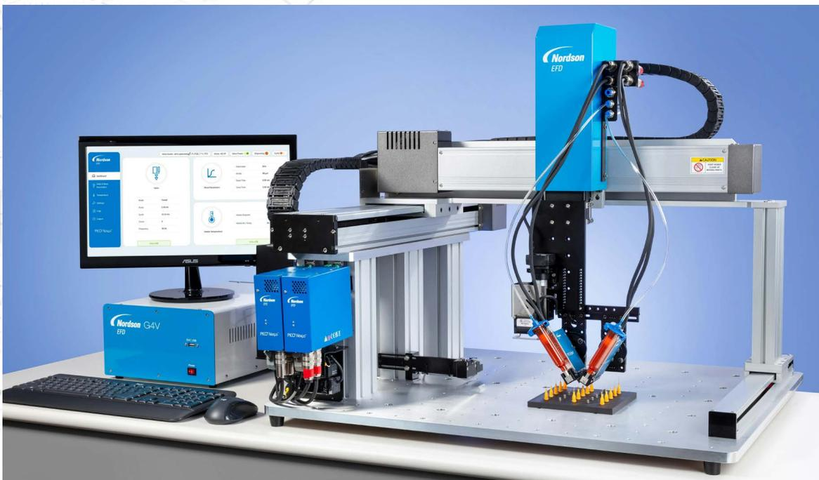
Two PICO NexuS jetting systems perform a needle-bonding application using a G4VPlus robot. The application is just one representation of Nordson EFD's smart factory and IIOT solutions.
