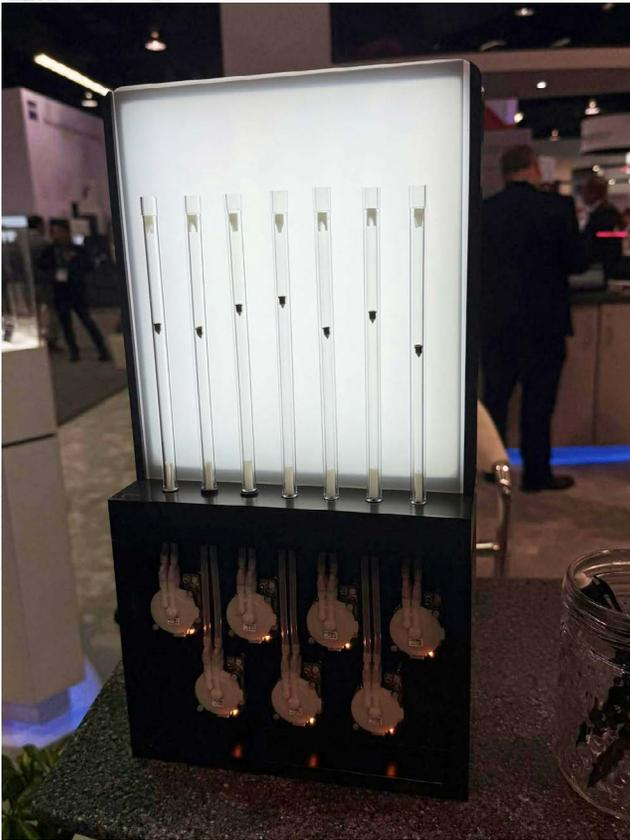
The Lee Company's newly acquired piezoelectric disc pump from Leventis is incredibly silent, pulsatile-free and compact, making it a suitable choice for a range of medical uses.
