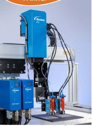
and other fluids used in assembly applications. The product has been certified for PROFINET devices and controllers, and ODVA (Open Device Vendor Association) has confirmed successful conformance testing for the Ethernet I/P protocol.
