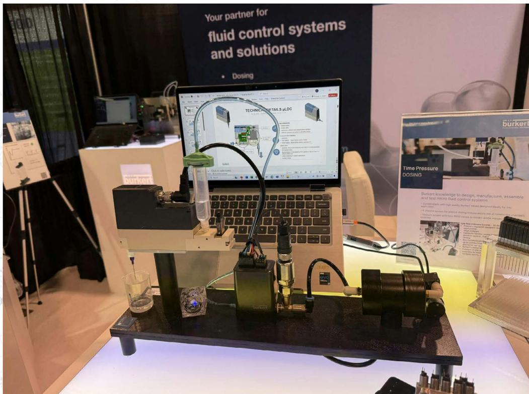
Burkert's liquid dosing system offers engineers in the medical device sector a solution for non-contact dosing with real-time feedback as well as accuracy.
