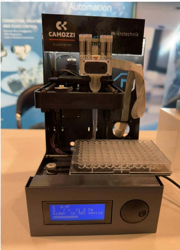
A specialized piezo pump, originally manufactured by Bartles, was modified by Camozzi's engineering team, culminating in the development of an advanced aspiration and dispense section, precisely crafted with the integration of solenoid valves, a manifold block and a custom-designed printed circuit board (PCB). Sharon Spielman/Machine Design
