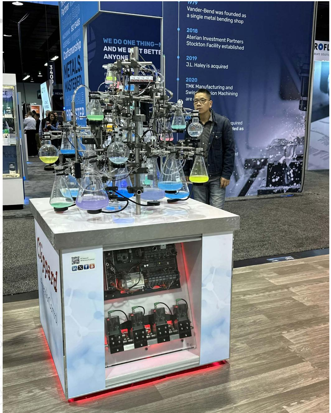
Clippard's pneumatic music machine was a showstopper. The contraption is constructed with different types of valves, as well as pressure controllers. Machine Design
