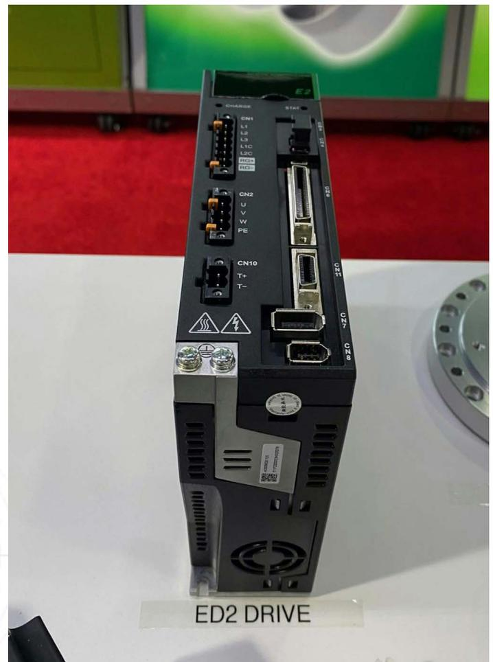
Integral to the performance of articulated and humanoid robots, HIWIN displayed their advancements in harmonic drive systems and strain wave bearings as well as its E2 drive, featuring embedded Ethernet IP protocol.
