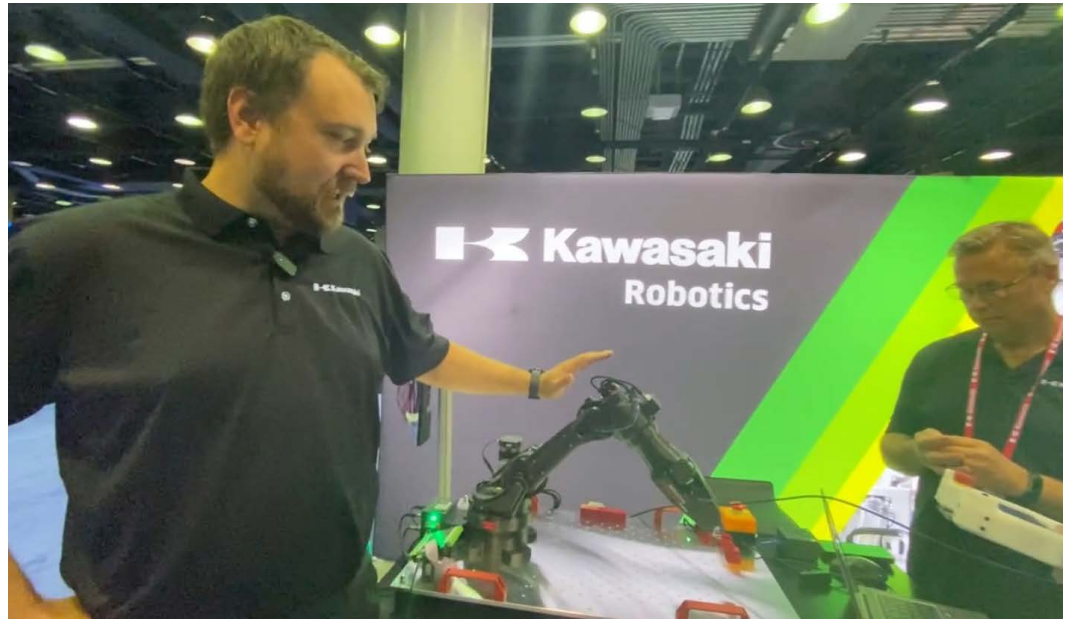
Cody Schenk, training instructor/developer at Kawasaki Robotics, demonstrates the company's educational 6-axis robot, the Astorino, which is 99.5% 3D printed.
