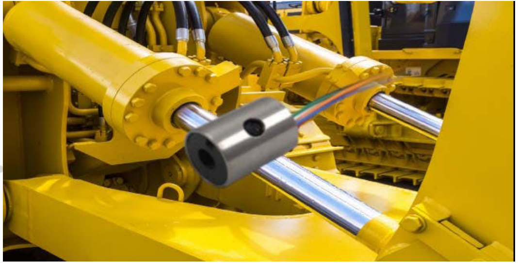
Figure 4: Vented LVDT sensors equalize pressure inside and outside the LVDT to operate reliably in temperature extremes of -65^{\circ}\text{F} to +400^{\circ}\text{F} and operating pressures of 30,000 psi. Offering a lightweight, low-mass core and a compact 3/8-in. diameter, these miniature AC-operated position sensors are ideal for high-response dynamic measurement.
