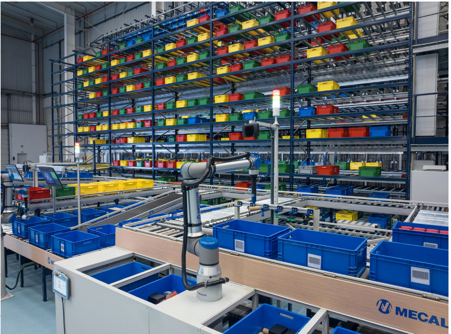
A new solution combining UR’s cobot arms with Siemens’ SIMATIC Robot Pick AI software and Zivid’s 3D sensors create a deep-learning picking solution for warehouse automation and intra-logistics fulfillment. Universal Robots
