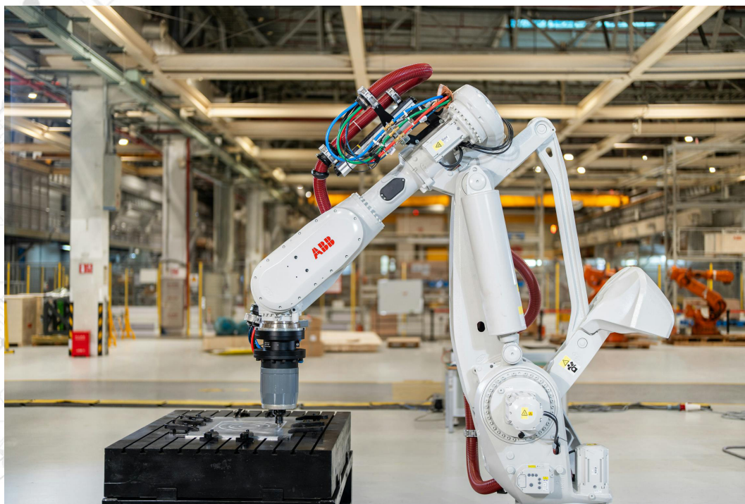
The IRB 7710's energy efficient design in combination with OmniCore's re-generation technology achieves up to a 30% energy reduction, according to ABB. ABB
