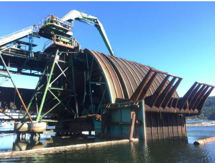
1. The arms that lift bundles of logs out of the bay and into the sawmill is operated by two 31-in.-long hydraulic cylinders.
