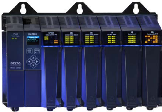
4. The RMC200 from Delta Computer Systems Inc. can control up to 32 motion axes simultaneously, plus it can serve as a data acquisition subsystem in test applications. A built-in Ethernet interface is provided for downloading motion programs or uploading motion status or test data from registers inside the controller.
