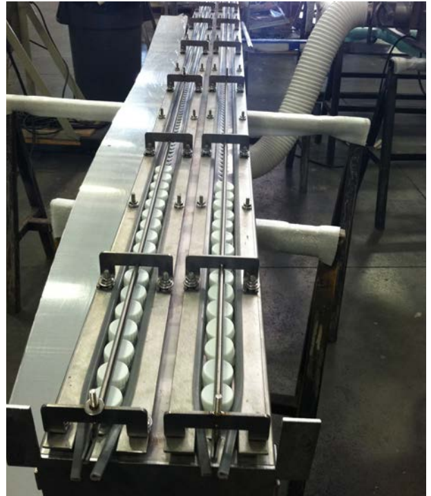
A dual-lane air conveyor uses a top bar cover to keep the bottle caps from leaving the line as they move along.
