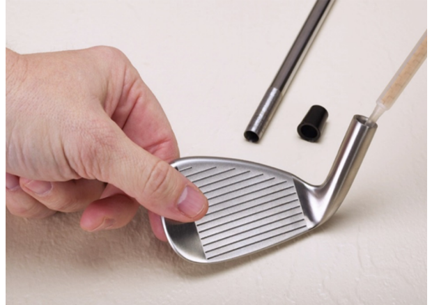
Bonding the shaft and hosel of a golf club with adhesives improves vibration resistance and impact strength.
