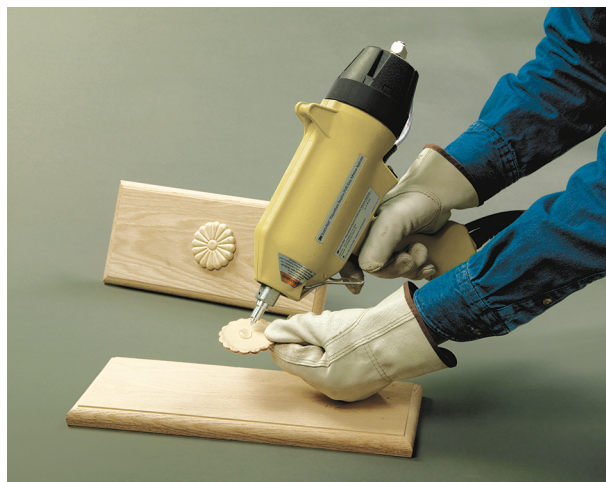
Mounting objects with adhesives or tapes allows for an invisible attachment and improved aesthetics to the overall design.
