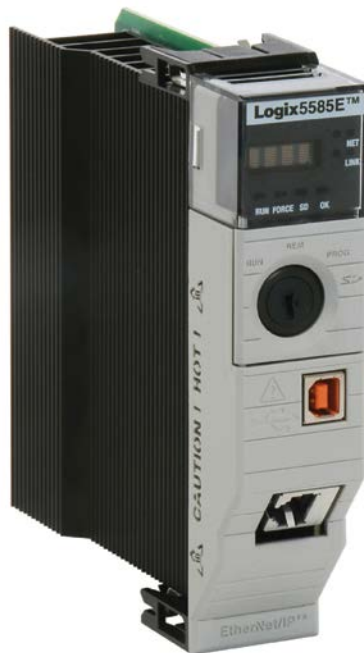
The Allen-Bradley ControlLogix 5580 controller includes an embedded 1-Gb Ethernet port to support high-performance communications, I/O, and applications with up to 256 axes of motion.
