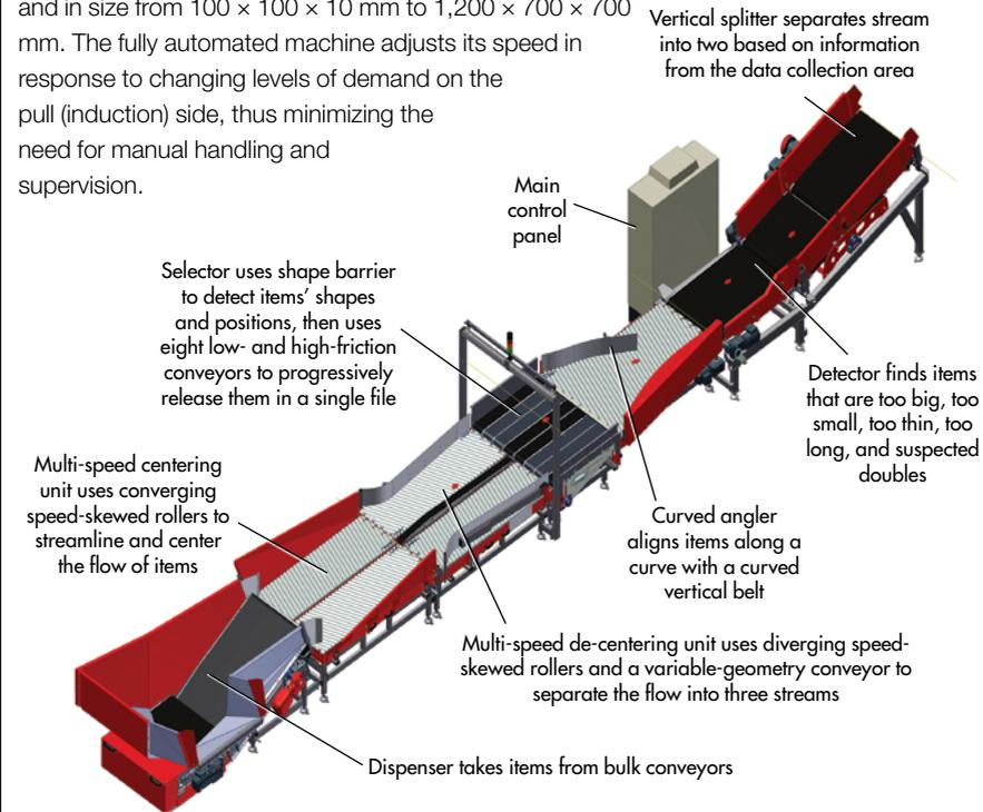
The machine uses a minimum of moving parts, so there is less wear and tear. Power-saving features, such as variable-speed drives and a sleep mode, save energy. The entire unit is controlled by PLCs. Frequency inverters let the machine recapture kinetic energy and convert it to electricity, minimizing its energy consumption.
